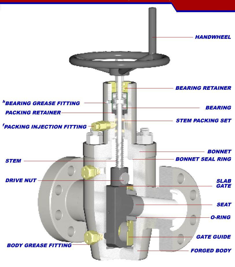
f) Stuffing box can be repacked via injectable packing while the valve is in service up to the rated working pressure.h) Valve bonnet equipped with grease port(s) and fitting(s) for bearing lubrication.
