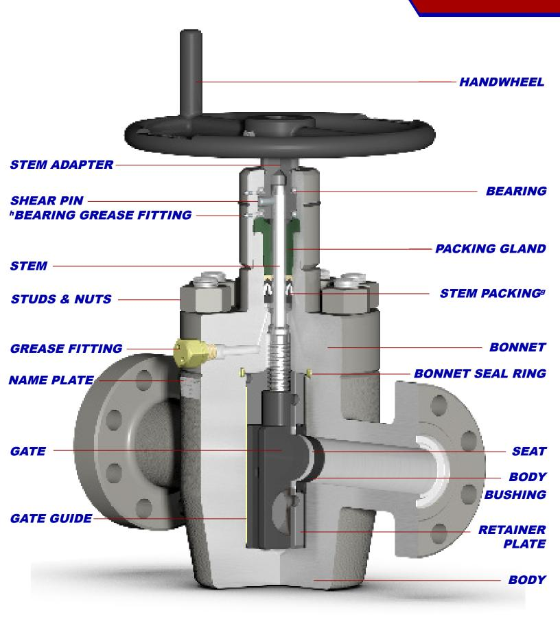
g) Stuffing box can be repacked via back seat while the valve is in service up to the rated working pressure.
