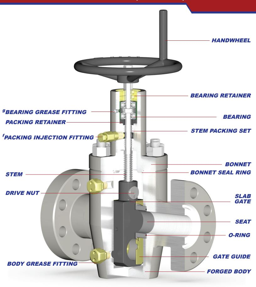
f) Stuffing box can be repacked via injectable packing while the valve is in service up to the rated working pressure.
