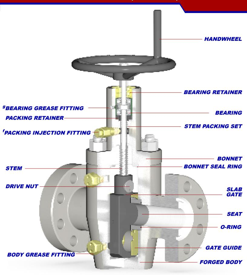
f) Stuffing box can be repacked via injectable packing while the valve is in service up to the rated working pressure.g) Valve bonnet equipped with grease port(s) and fitting(s) for bearing lubrication.
