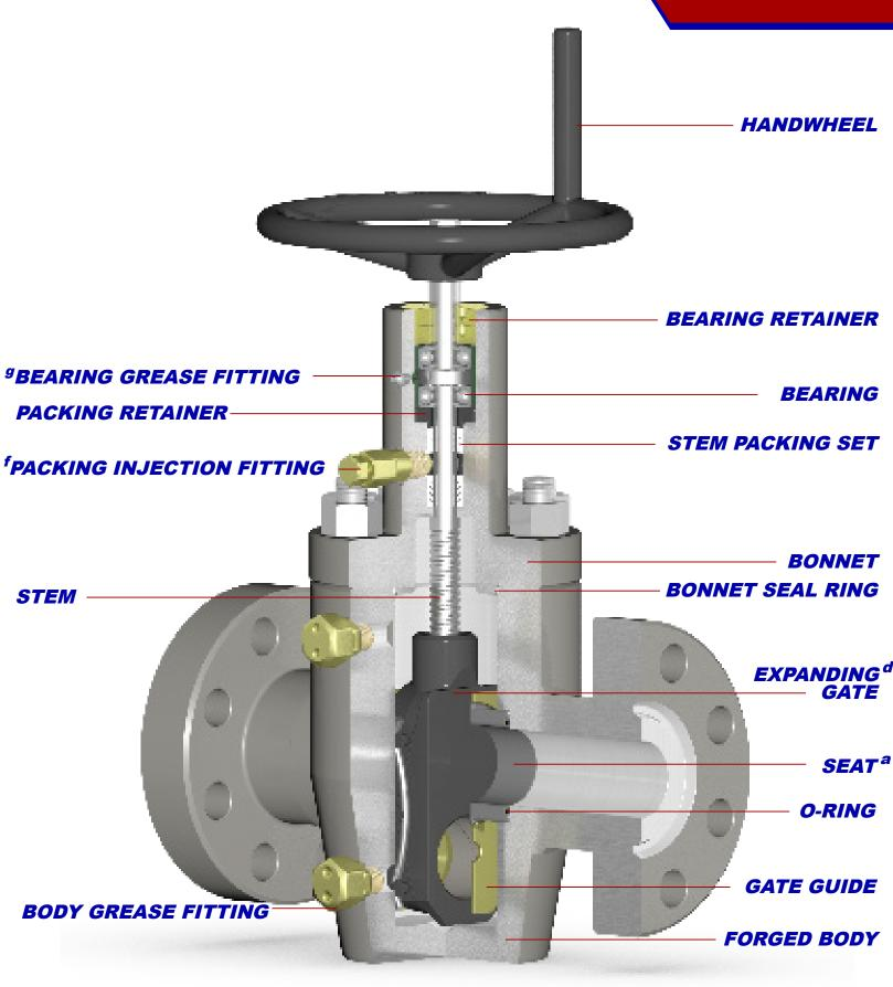
a) Equipped with a non-sealing seat on the upstream side. See engineering note titled "Model MDS (Model M Directional Seal)" for details.
